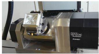
"KME CNC designed its newest addition to its line with the traditional approach in mind: how to be more efficient with what you currently have," said a company spokesperson. Due to its compact size, the 5-axis trunnion design will allow the operator to integrate the table on virtually any machine, i.e no size restriction. Constructed similarly to the larger trunnions, this unit is built out of Meehanite cast iron and billet aluminum covers and provides the same benefits.
