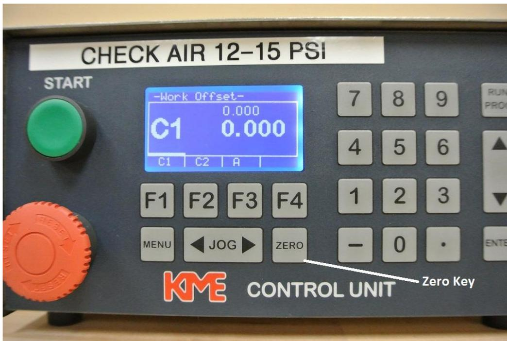
**6)** Now, the control box is ready for use. To start cutting parts, simply push the “START” button on the left side of the control box to bring the KME system in DPRNT mode. The screen will read “DPRNT” on the top left corner (as shown below), confirming that your KME system is now ready to receive DPRNT commands from your VMC. If you would like to exit DPRNT mode, push e-stop and it will allow you to exit DPRNT mode.
