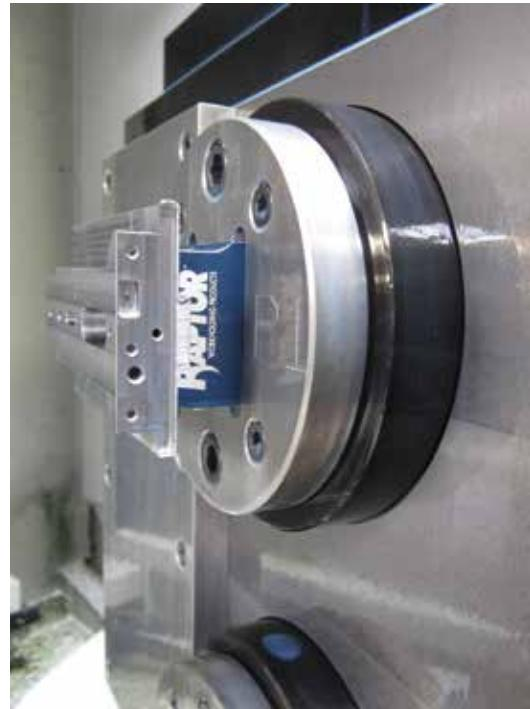
to provide the fifth axis of movement atop the HMC's fourth-axis table, which would enable the shop to benefit from a 3+2 positioning style of five-axis machining.
