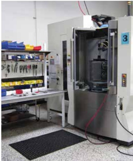
The HMC's 160-station ATC magazine enables the shop to keep a number of standard tools installed inside the machine at all times while establishing a tool database inside its CAM software. If no special tools are required for a job, setup time is effectively zero.
