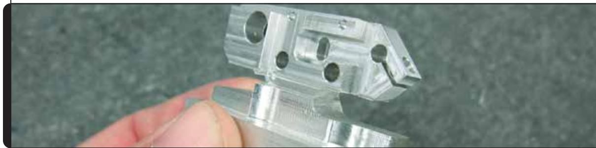
Campbell Engineering benefits from a new twist on the tombstone workholding concept, which enables one of its HMCs to perform 3+2 machining to reduce scrap while supporting the higher-volume needs of its medical customers.
