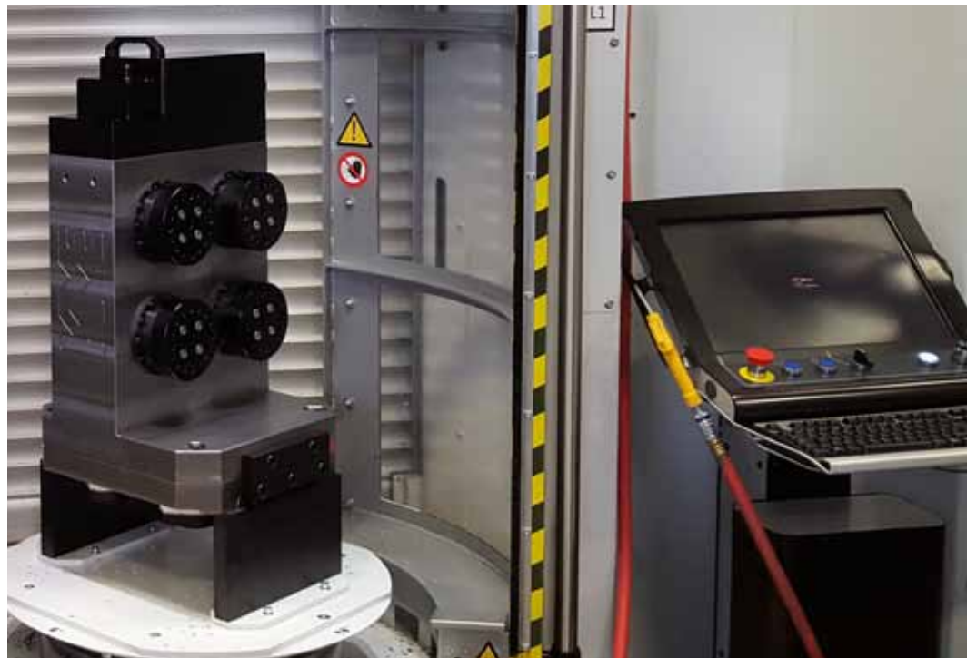
KME CNC's Wireless Tombstone in a Pallet Pool Application
